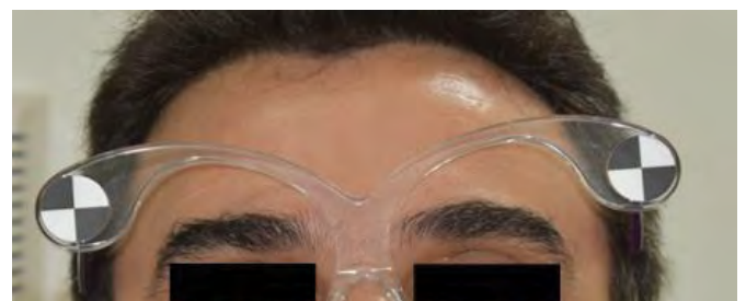
Figure 2 The digital calibrating goggle provided with DSS software.
