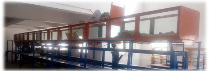
Figure 1: Shape of the experimental wave flume
