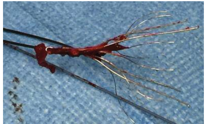
Figure 4. IVC filter after removal with bent prongs.
