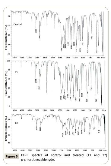
to peaks at 1093-1207 cm<sup>-1</sup> region of spectra in all three samples; whereas, the in-plane deformation was assigned to peaks in the range of 702-839 cm<sup>-1</sup> (control), 704-839 cm<sup>-1</sup> (T1), and 704-837 cm<sup>-1</sup> (T2) sample.
