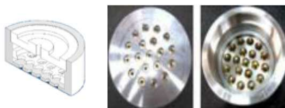
Fig.2 Internal and external scheme of the circular injector plate
