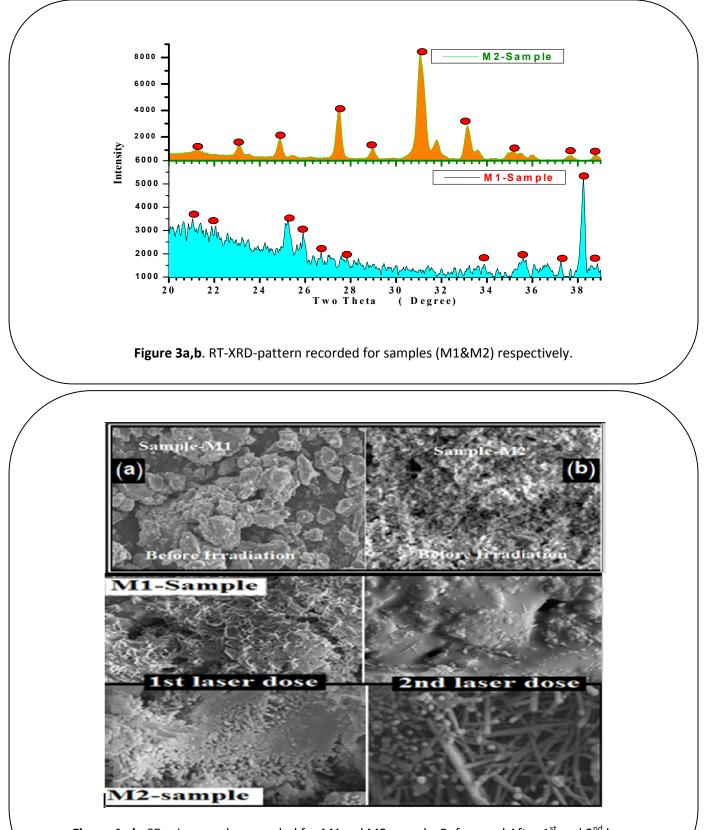
**Figure 4a,b**. SE-micrographs recorded for M1and M2-samplesBefore and After 1<sup>st</sup> and 2<sup>nd</sup> laser irradiation dose.
