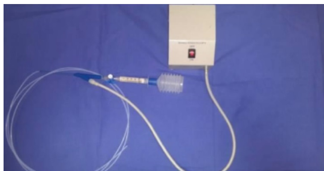
Figure 1 Haemoseal Spray Kit with air pump, Haemoseal probe, a 7.5 Fr spray catheter, 230 cm in length (Shaili Endoscopy, India) and collagen cartridge.
