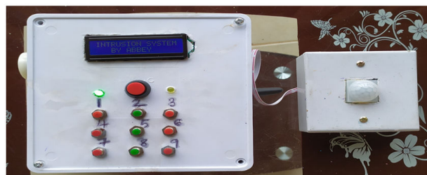
Figure 14: External view of the intrusion detection and alert system.
