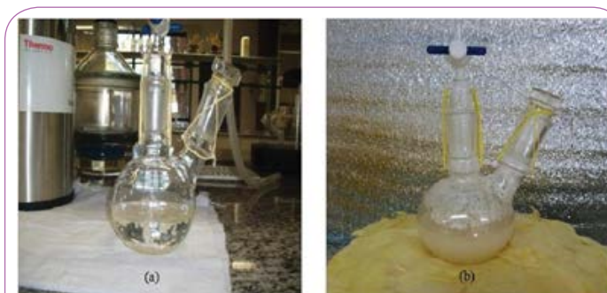
Figure 1 Homogeneous solution of PA66 in HC after testing affinity between components with spontaneous solution formation.
