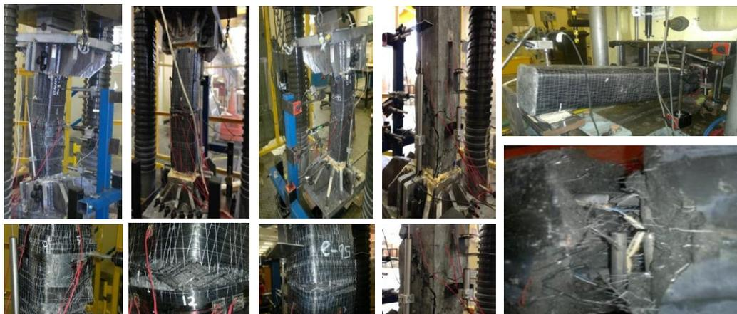
**Figure 4** Typical failure modes of UHPC-filled FRP tube specimens and unconfined UHPC columns.
