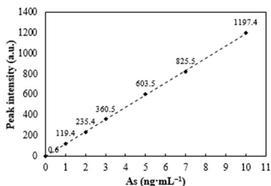
**Figure 2:** Calibration curve for the determination of total As
