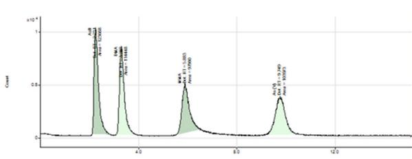
**Figure 3:** Chromatographic separation of arsenic standards at 10 ng.g<sup>-1</sup>
