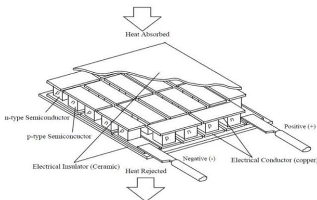
**Figure 1:** Construction of a typical thermoelectric module.
