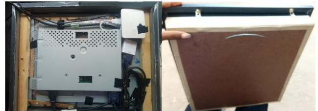
Figure 9: Image showing the internal view of the digital photo frame and after covering, ready for hanging
