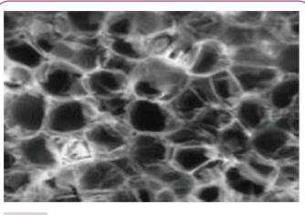
Figure 3 Typical microstructure of layer I of corncob in 400  $\mu$ m.
