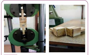
Figure 11 Test setup of IB test MC particle board.
