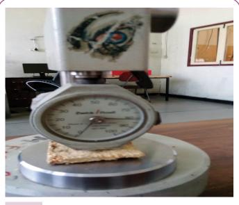
Figure 12Hardness measuring setup of particle board.
