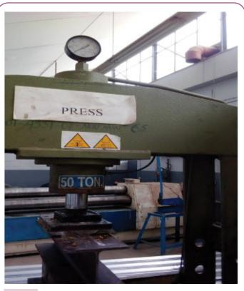
Figure 8 Manually hydraulic press machine.
