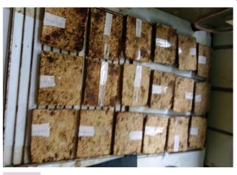
Figure 10 Experimental products of maize cob particle board.
