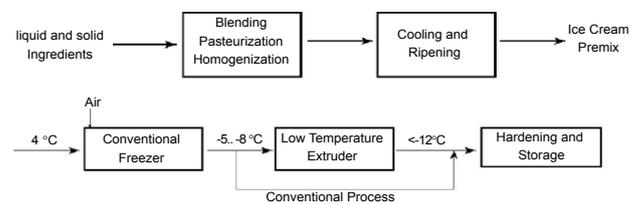
**Figure 1** Flow chart of combined continuous freezer and LTE process of ice cream manufacturing.
