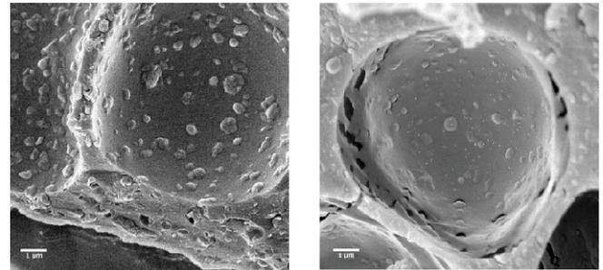
**Figure 6** LEFT: Cryo-SEM image of SS-LTE showing more aggregate fat particles over bubble surface. RIGHT: Cryo-SEM image of TS-LTE showing less aggregated fat particles over bubble surface.
