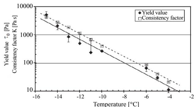
**Figure 3** Graph of yield value  $\tau_0$  and consistency factor  $K$  as a function of temperature.
