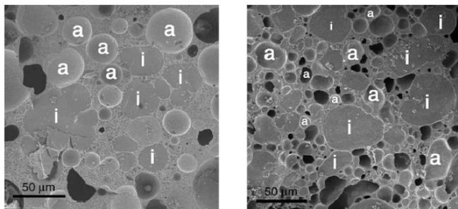
**Figure 5** Cryo-SEM analysis of ice cream. (Left) Image of ice cream processed in convention freezer at drawing temperature of  $-4.7^\circ\text{C}$  (Right) Image of ice cream processed in combined freezer / LTE system at drawing temperature of  $13^\circ\text{C}$  (i) ice crystals (a) air cells.
