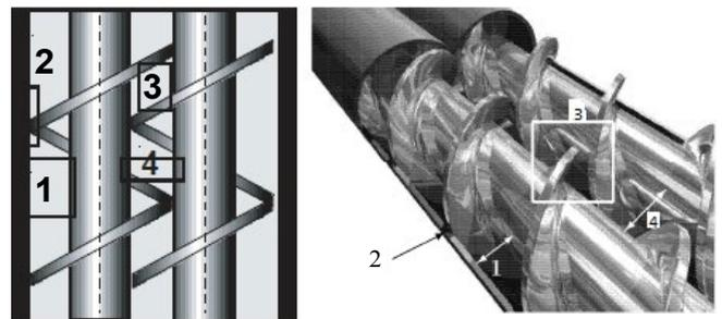
**Figure 2** Shear zones in TS-LTE: Screw channel gap (zone 1), clearance gap (zone 2), tangential gap (zone 3) and screw roots gap (zone 4).
