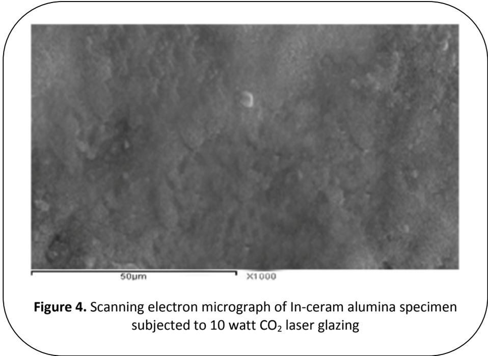
**Figure 4.** Scanning electron micrograph of In-ceram alumina specimen subjected to 10 watt CO<sub>2</sub> laser glazing
