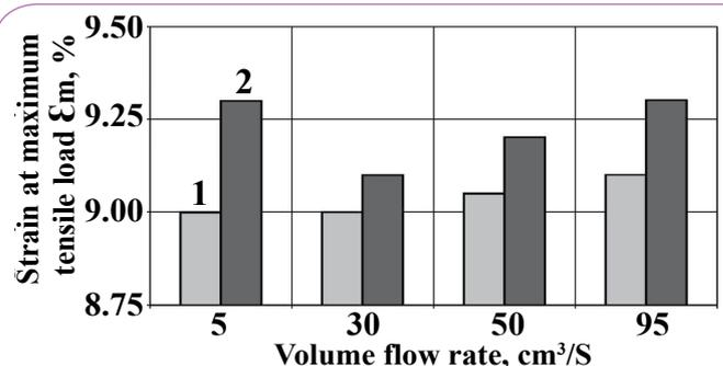
**Figure 12** Relationship between strain at maximum tensile load and volume flow rate of: 1 – unfilled polymer, 2 – polymer containing 10% glass powder.
