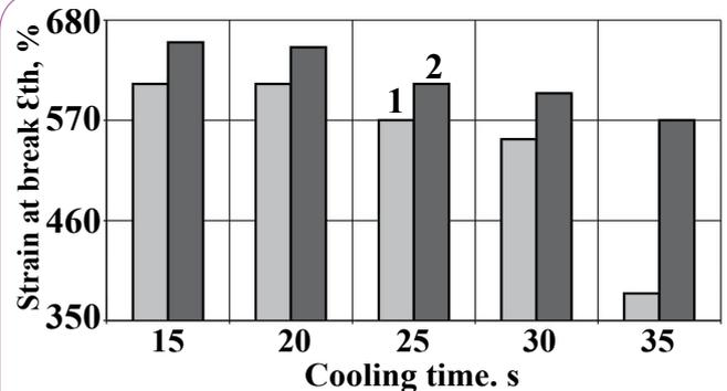
**Figure 6** The relationship between strain at break and cooling time of parts moulded from polyethylene GD 7255: 1 – unfilled with glass powder, 2 – filled with (10%) glass powder.
