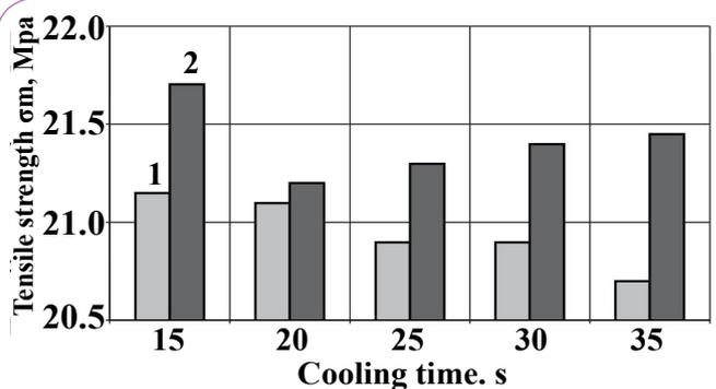
**Figure 5** The relationship between tensile strength and cooling time for 1 – parts injection moulded from unfilled polyethylene GD7255, 2 – injection moulded parts filled with (10%) glass powder.
