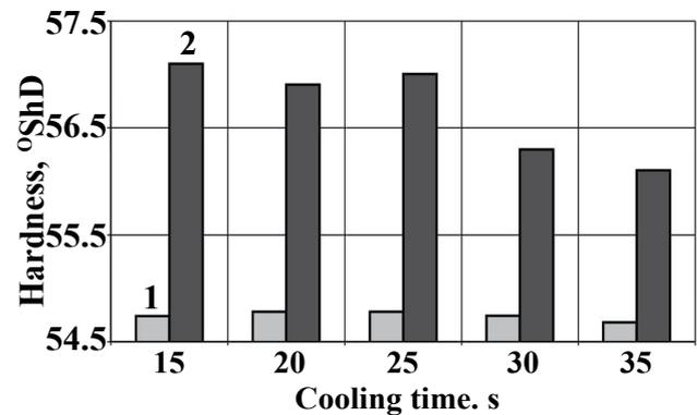
**Figure 3** The relationship between hardness and cooling time of parts moulded from polyethylene GD 7255: 1 – unfilled 2 – filled with (10%) glass powder.
