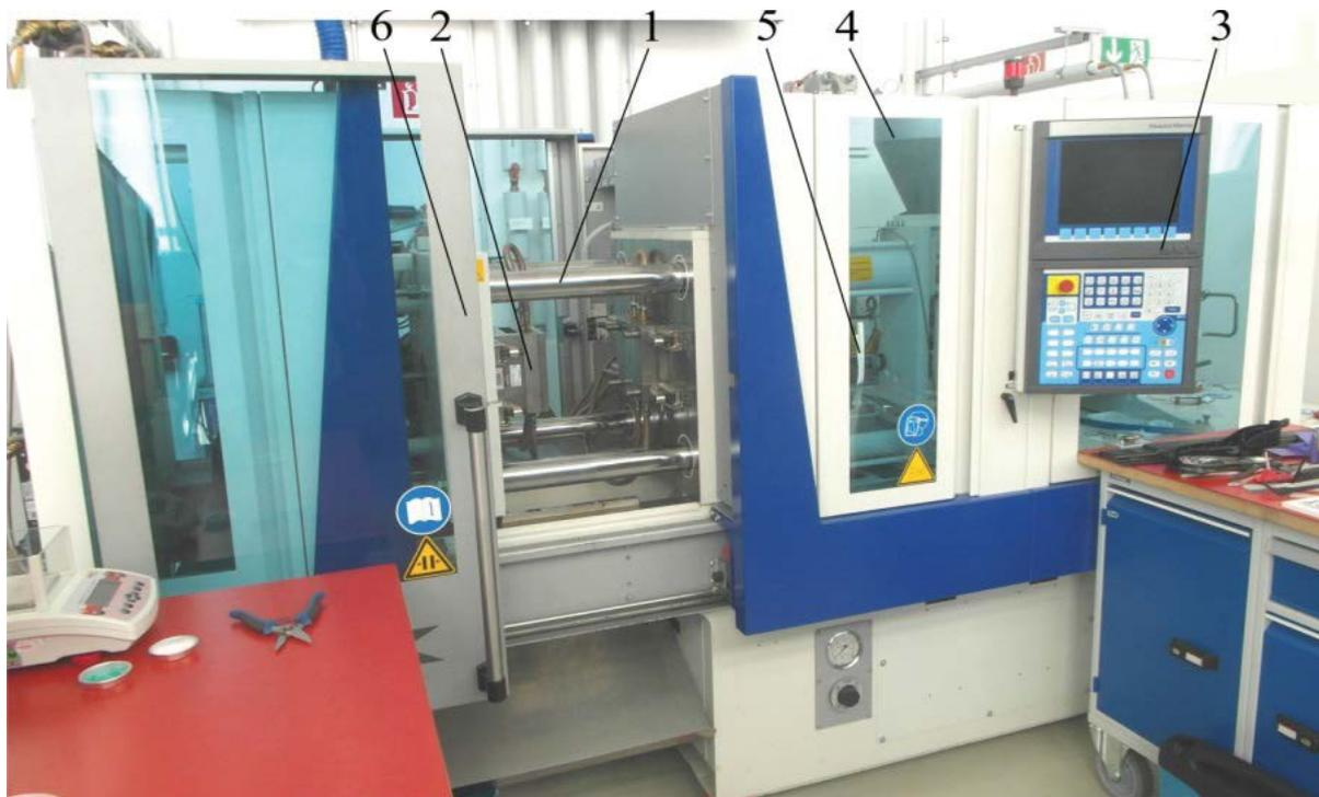
**Figure 2** View of the Krauss Maffei KM 50-55CX injection moulding machine: 1 – runner, 2 – injection mould, 3 – control panel, 4 – hopper, 5 – plasticizing system, 6 – movable door of the tool system.
