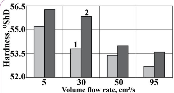
**Figure 8** The dependence of hardness on volume flow rate for: 1 – unfilled polymer, 2 – polymer containing 10% of glass powder.
