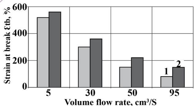
**Figure 11** Strain at break as a function of volume flow rate for: 1 – unfilled polymer, 2 – polymer containing 10% of glass powder.
