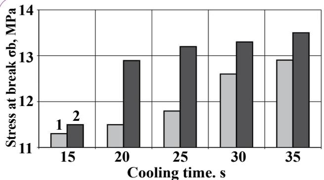
**Figure 4** Stress at break as a function of cooling time of: 1 – unfilled injection moulded parts 2 – injection moulded parts filled with (10%) glass powder.
