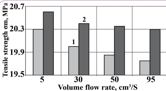
**Figure 10** The relationship between tensile strength and volume flow rate for: 1 – unfilled polymer, 2 – polymer containing 10% glass powder.
