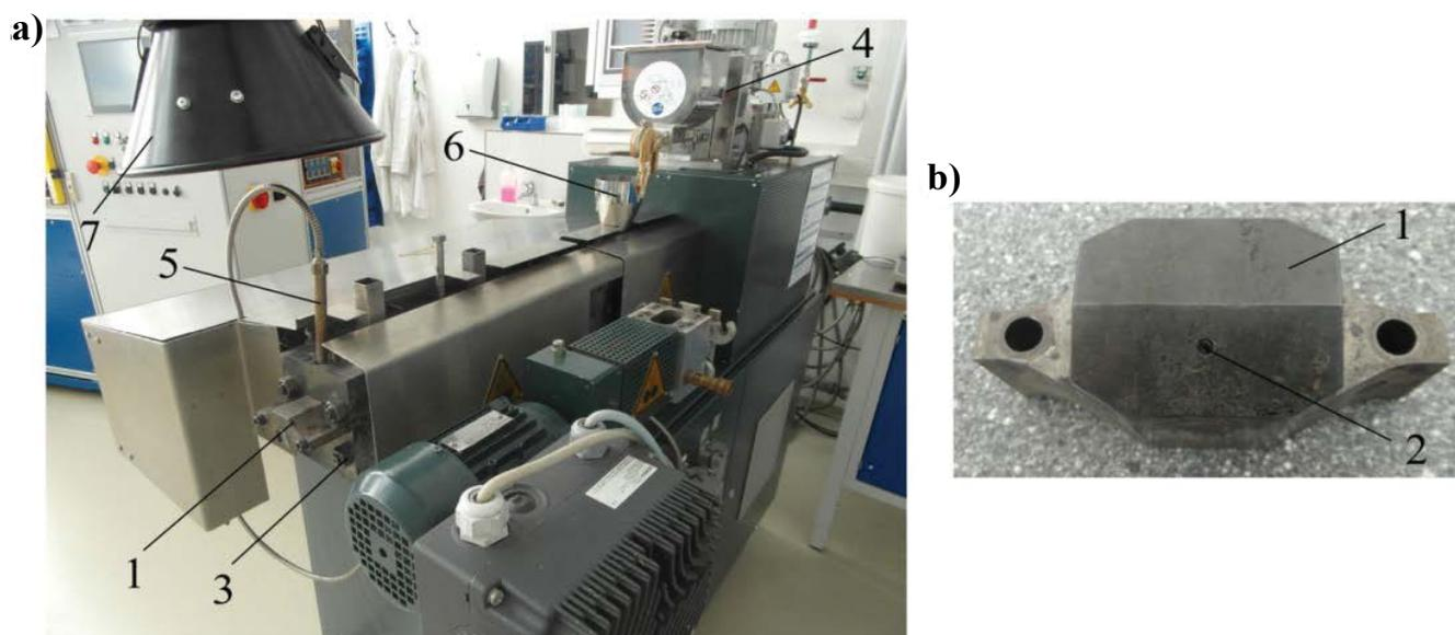
**Figure 1** View of the ZSK 18 MEGAlab twin-screw extruder and the extrusion head with a circular cross-section die: 1 – extrusion head, 2 – die, 3 – plasticizing system, 4 – feeder, 5 – pressure and temperature sensor, 6 – hopper, 7 – ventilating hood.
