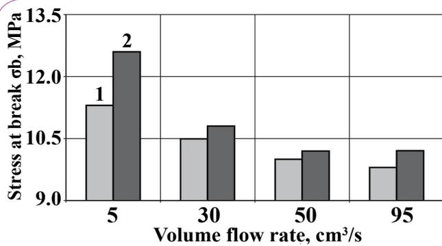
**Figure 9** The dependence of stress at break on volume flow rate for: 1 – unfilled polymer, 2 – polymer containing 10% glass powder.
