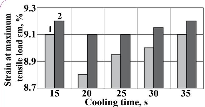
**Figure 7** The dependence of strain at maximum tensile load on cooling time of parts moulded from polyethylene GD 7255: 1 – unfilled with glass powder, 2 – filled with (10%) glass powder.
