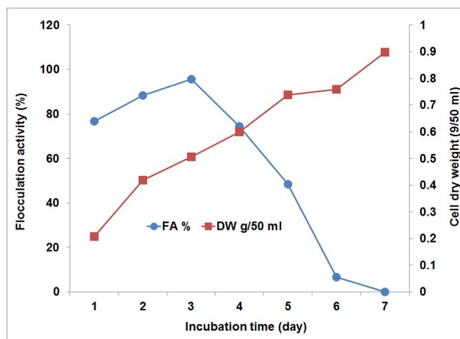
Figure 4: Time course of growth and bioflocculation activity of strain DFH1 (clay concentration =5g/L, agitation speed= 2min at 230rpm then 3min at 80 rpm, dosage of strain supernatant = 2.5ml/L, dosage of CaCl<sub>2</sub> (3%) = 50ml/L clay suspension pH=7)
