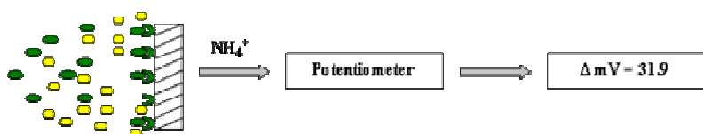
a. Control (without inhibitor) urease act on substrate to produce NH 4 + ions sensed by ISE
