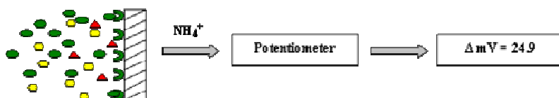
b. Reaction in presence of inhibitor at low concentration showing decrease in change in potential
