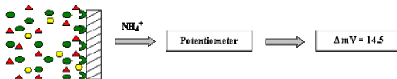
c. Reaction in presence of inhibitor at higher concentration showing further decrease in change in potential
