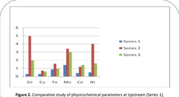
Discharge point (Series 2) and Downstream (Series 3) water samples
