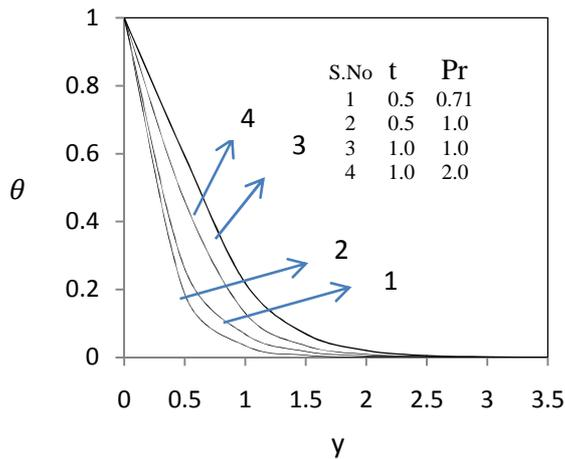
Fig 5(c): Temperature profiles for different values of **Pr & t** with **a=0.1**.
