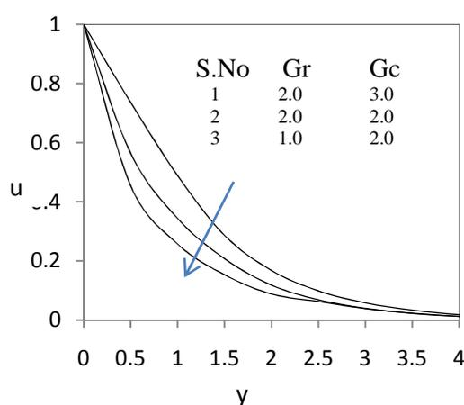
Fig.1 (c): Velocity profiles for different values of  $Gr$  and  $Gc$  with  $\alpha=1, a=0.1, Pr=0.71, Sc=0.22, t=0.5$
