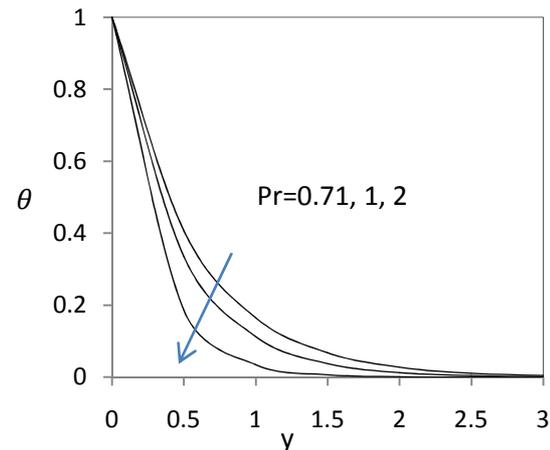
Fig.5 (b): Temperature profiles for different values of  $Pr$  with  $a=0.1, t=0.5$
