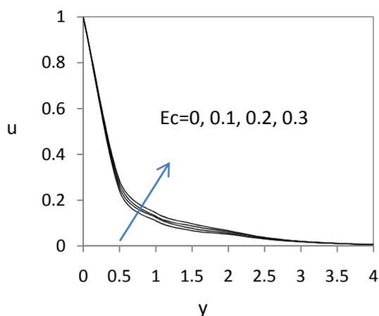
Fig 2(a): Velocity profiles for different values of  $Ec$  with  $a=0.1, Pr=0.71, Sc=0.22, Gr=1.0, Gc=1.0, \alpha=1, t=0.5$
