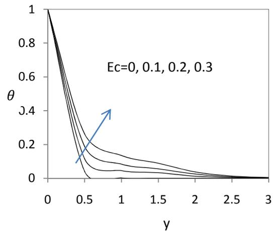
Fig 5(d): Temperature profiles for different values of **Ec** with **Pr=2.0, a=0.1, t=0.5**.
