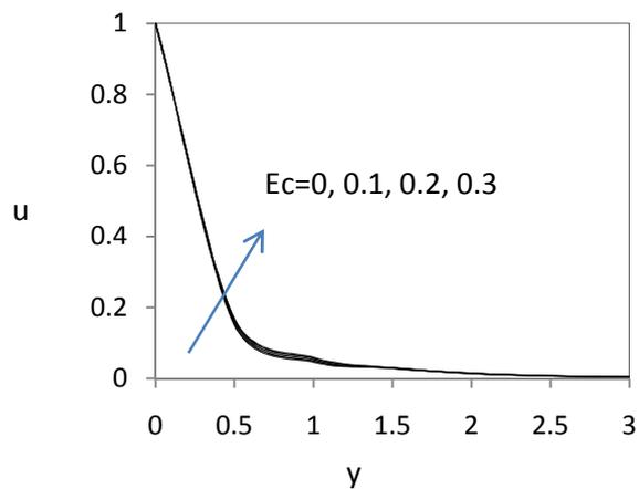
Fig 2(b): Velocity profiles for different values of  $Ec$  with  $a=2.0, Pr=0.71, Sc=0.22, Gr=1.0, Gc=1.0, \alpha=1, t=0.5$
