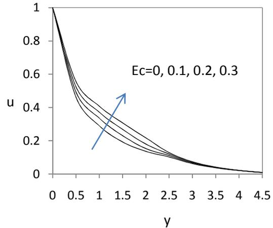
Fig 3(b): Velocity profiles for different values of  $Ec$  with  $\alpha=-1$ ,
