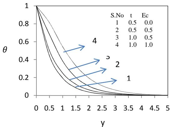
Fig 5(e): Temperature profiles for different values of **Ec & t** with **a=0.1, Pr=0.71**.
