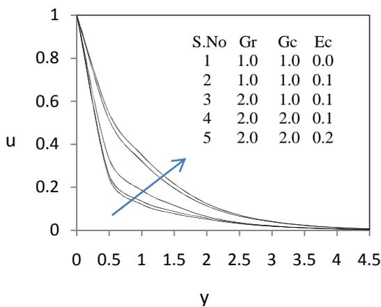
Fig 4(a): Velocity profiles for different values of  $Ec, Gr \& Gc$
