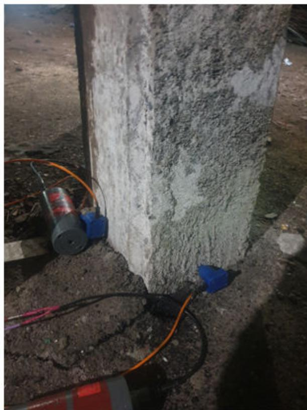
Figure 4: Example of installation of horizontal and vertical geophones gs20dx and single-channel digital recorders Texan (RefTek-125A) on piles.
