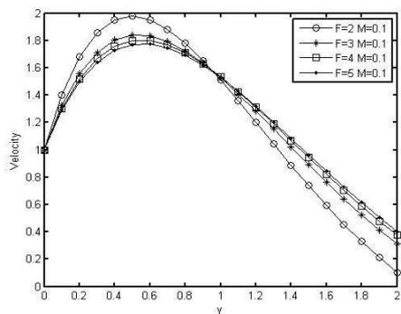
Fig.3: Effect of F on the velocity field.
