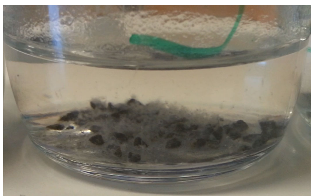
Figure 2: Greyish precipitates formed during water treatment for As(V) removal using mixed oxidation state manganese compound \text{Mn}_8\text{O}_{10}\text{Cl}_3 -modified clinoptilolite zeolite.
