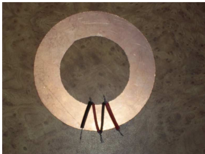
Fig 6 Thermocouples mounted on the GPB
