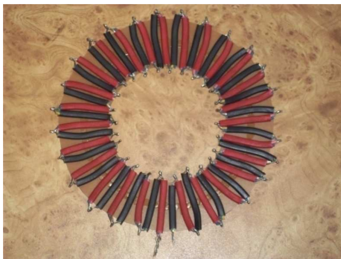
Fig 7 Completely fabricated thermopile mounted on the hollow GPB
