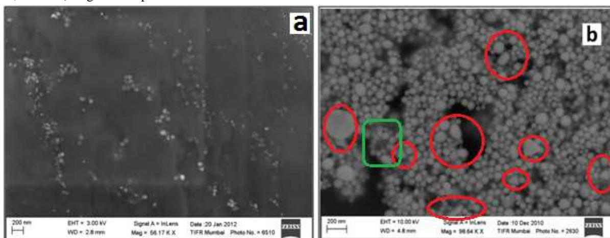
**Figure – 4:** FEG SEM image exhibiting the impact of temperature and pH on the biosynthesis of gold nanoparticles using *A. racemosus* (a) pH8 at 30°C (b) pH2 at 100°C. Red circles show the presence of non-spherical gold nanoparticles such as triangles, oval and hexagonal shaped. Green box demonstrate the formation of a unique ring of spherical gold nanoparticles.
