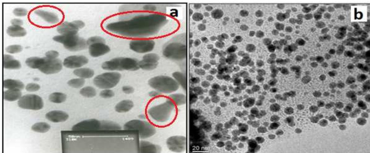
**Figure-5: TEM image of gold nanoparticles synthesised using *A.racemosus* showing the impact of concentration of gold salt and temperature (a) 150ppm gold salt at pH 8 at 100 ° C(b) 37°C at pH 8 and 100 ppm gold salt**
