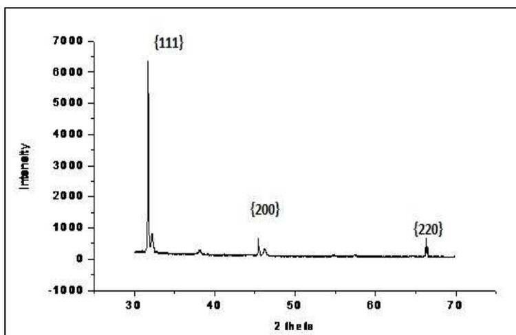
**Figure- 6: XRD pattern of gold nano particles synthesized using leaf extract of *Asparagus racemosus*, showing typical Bragg reflections for gold nanoparticles**
