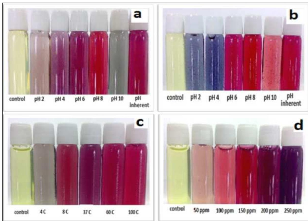
**Figure-1: Visual observation of temperature, pH and concentration on bio-fabrication of gold nanoparticles using *A. racemosus*, (a) impact of 30°C & different pH values (b) Impact of 100°C & different pH values. (c) Impact at pH 8 at various temperatures (d) impact at 100°C and pH 8 at various temperatures**
