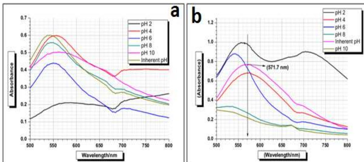
**Figure-2: Impact of temperature and pH on bio-fabrication of gold nanoparticles using *A. racemosus*, as shown by UV-Vis Spectroscopy (a) impact of 30°C & different pH values (b) impact of 100°C & different pH values. The inset shows the change in SPR with respect to different parameter**
