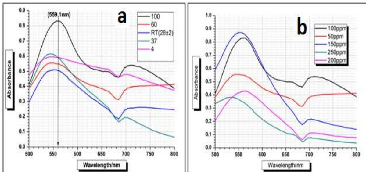
**Figure- 3:** UV-Vis spectra of gold nano particles biosynthesized at pH 6 using leaf extract of *A. racemosus* at (a) Different temperatures and (b) Different concentrations of aurochlorate
