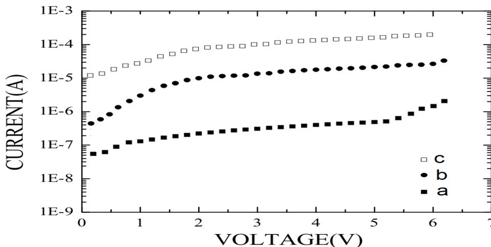
Figure5 I-V characteristics of porous silicon (a)before irradiation (b)after 50Gy gamma irradiation (c) after 100Gy gamma irradiation
