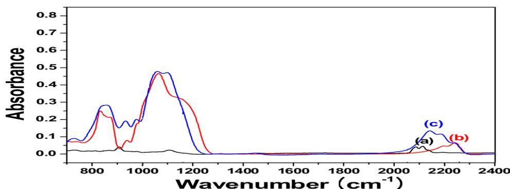
Figure 3 FTIR spectrum for PSi (a) before irradiation (b) after 50 Gy gamma irradiation (c) after 100 Gy gamma irradiation
