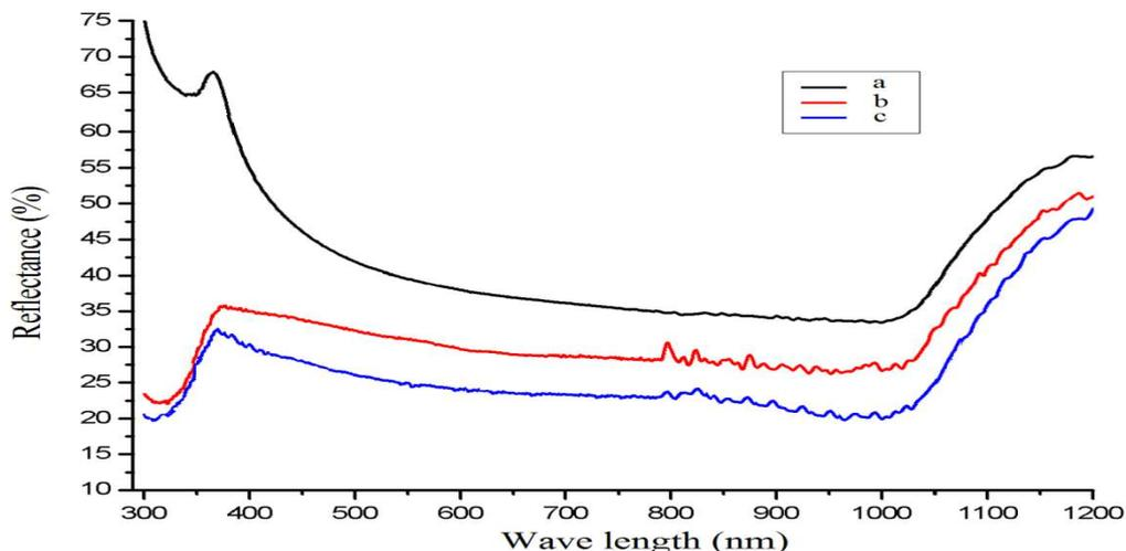
Figure4 reflectivity spectrum for PSI (a)before irradiation (b)after 50Gy gamma irradiation (c) after 100Gy gamma irradiation
