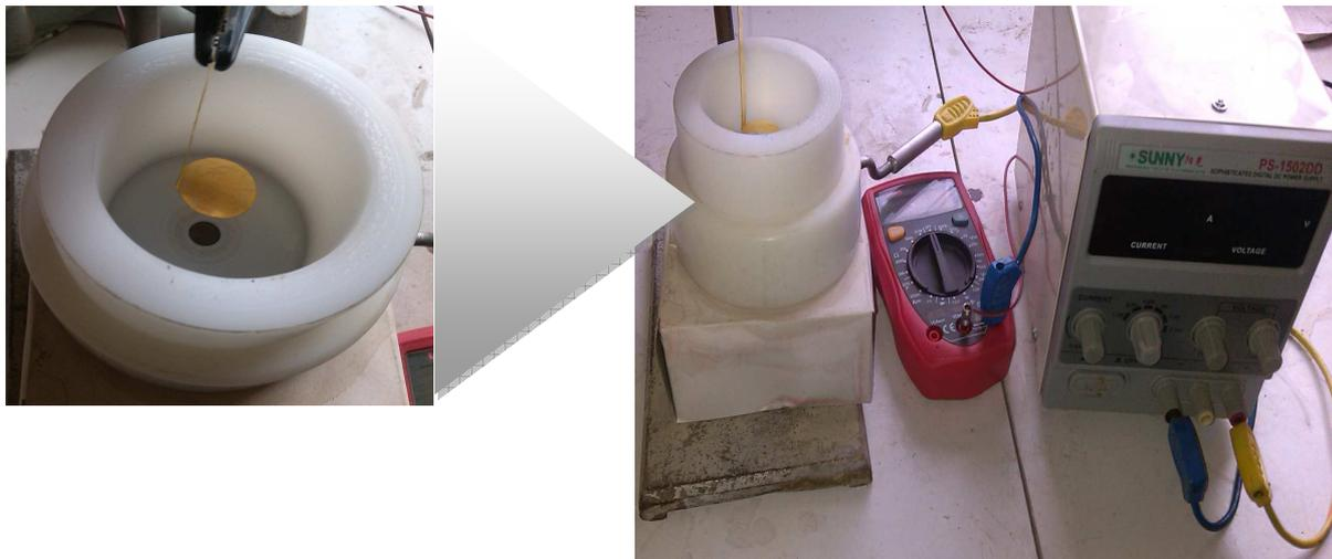
Figure 2 shows image of the electrochemical cell used in the sample preparation
