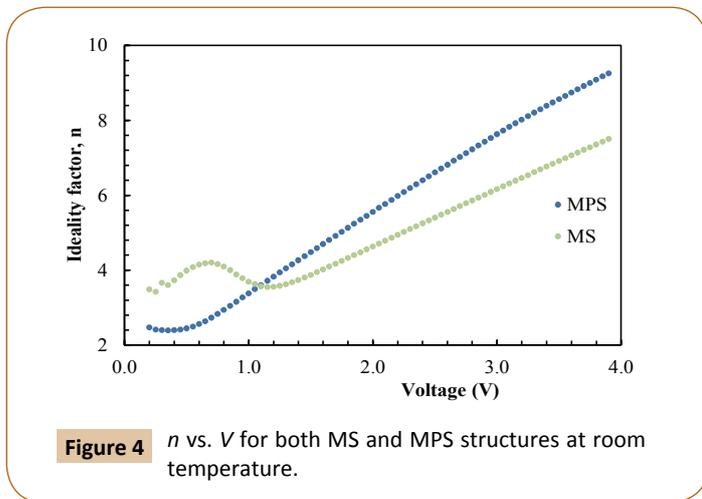
**Figure 4** n vs. V for both MS and MPS structures at room temperature.
