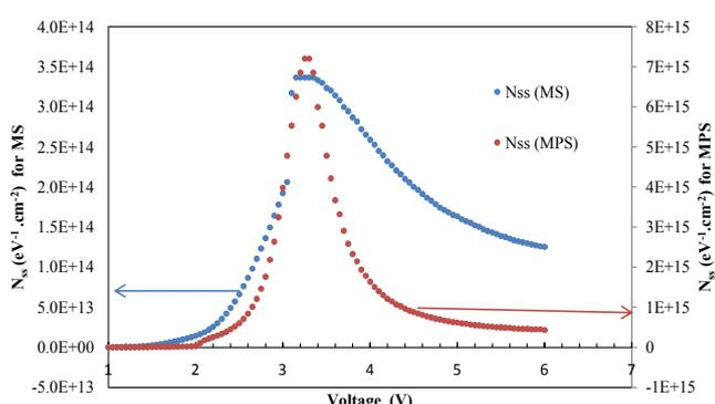
**Figure 12** Profiles of  $N_{ss}$  vs.  $V$  for the MS and MPS structures obtained by the high-low frequency capacitance method at room temperature.
