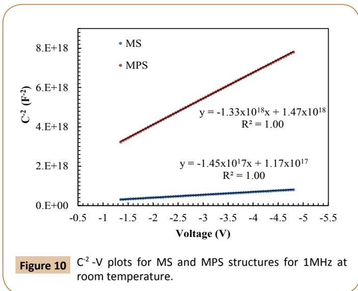
**Figure 10**  $C^2$ -V plots for MS and MPS structures for 1MHz at room temperature.
