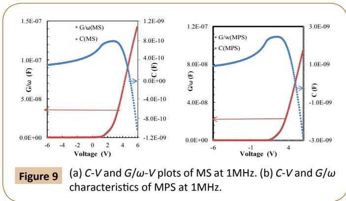
**Figure 9** (a) C-V and  $G/\omega$ -V plots of MS at 1MHz. (b) C-V and  $G/\omega$  characteristics of MPS at 1MHz.
