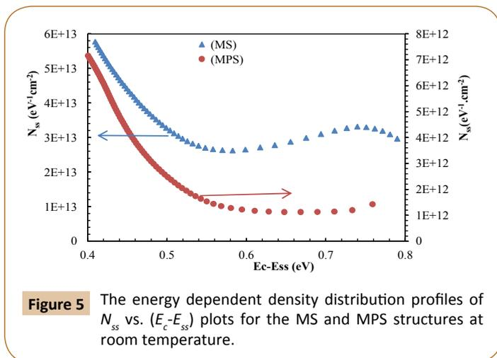
**Figure 5** The energy dependent density distribution profiles of  $N_{ss}$  vs.  $(E_c - E_{ss})$  plots for the MS and MPS structures at room temperature.
