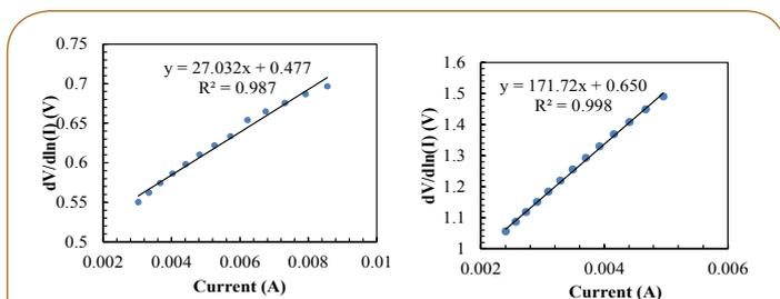
**Figure 6** (a)  $dV/d\ln(I)$  vs. I for MS structure. (b)  $dV/d\ln(I)$  vs. I for MPS structure.
