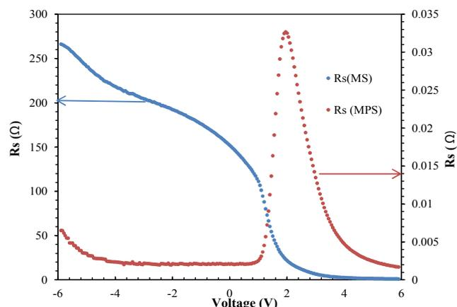
**Figure 11**  $R_s$  vs.  $V$  plots of the MS and MPS structures for 1 MHz at room temperature.
