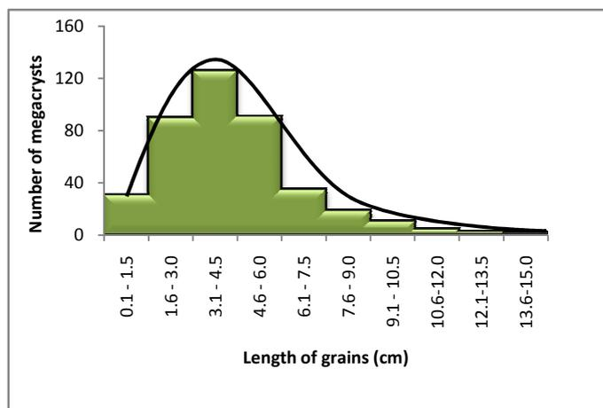
**Fig. 4a:** 3.1 – 4.5 (cm) is the highest frequency of grain lengths of the megacrysts; megacrysts frequency increases until megacrysts length reaches a maximum at 3.1-4.5 cm. After that megacrysts frequency decreases with increase in length
