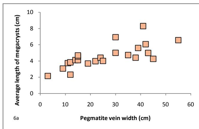
**Fig. 6a the average length of the megacrysts in each vein increases as the pegmatite vein sizes increase**
