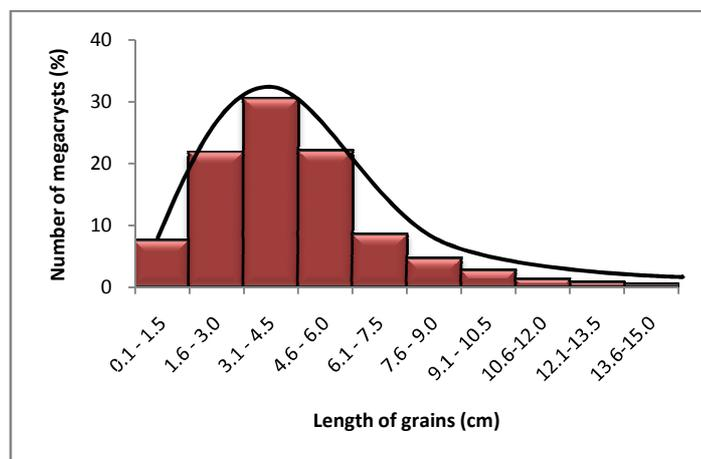
**Fig. 4b:** the megacrysts vary in frequency (%) with increase in grain length; megacrysts frequency increases until megacrysts length reaches a maximum at 3.1-4.5 cm. After that megacrysts frequency decreases with increase in length.
