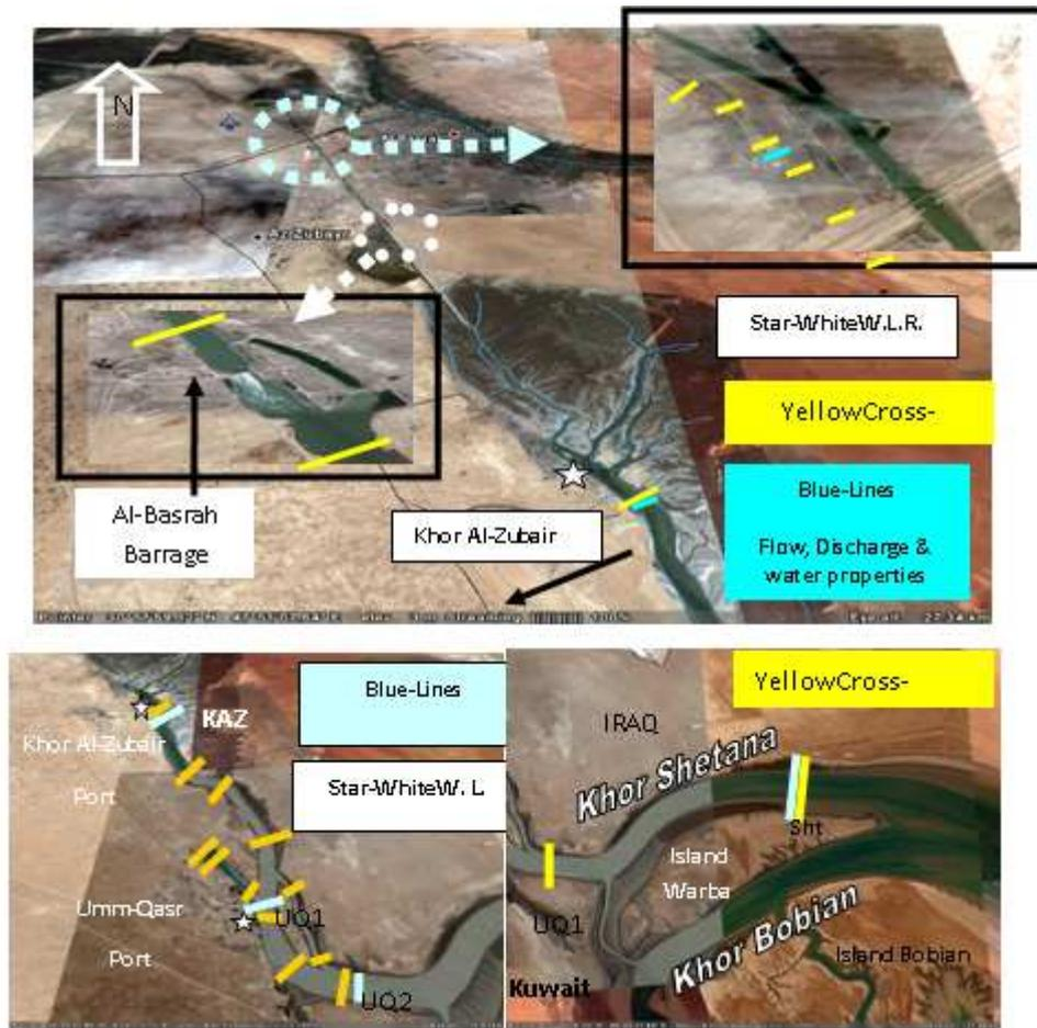
**Figure 5. Satellite image showing approximate Locations of the selected cross sections in Shatt Al-Basrah canal and Khor Al-Zubair to be measured (depth, position, water level, water properties, discharge, speed, and direction)**
