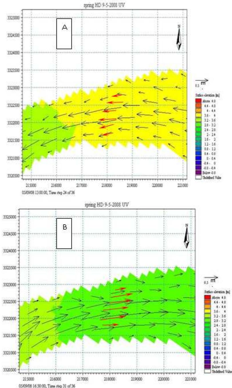
**Figure 9. Simulation (black arrow) and measurements (red arrow) of currents in Khor Shetana during the spring tide phase on 9-5-2008 A-flood B-ebb**
