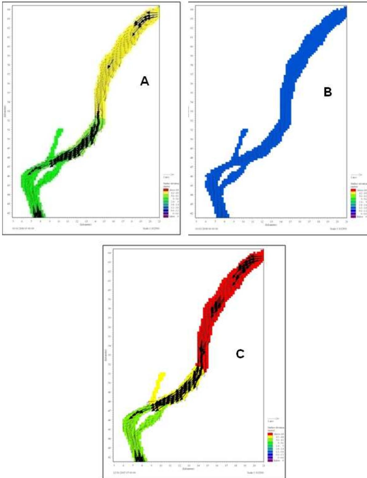
Figure 11. Tidal currents field in surface layer (surface currents) of the KAZ at the neap phase from 31-12-2007 to 1-1-2008: A-Flood B-Slack C-Ebb
