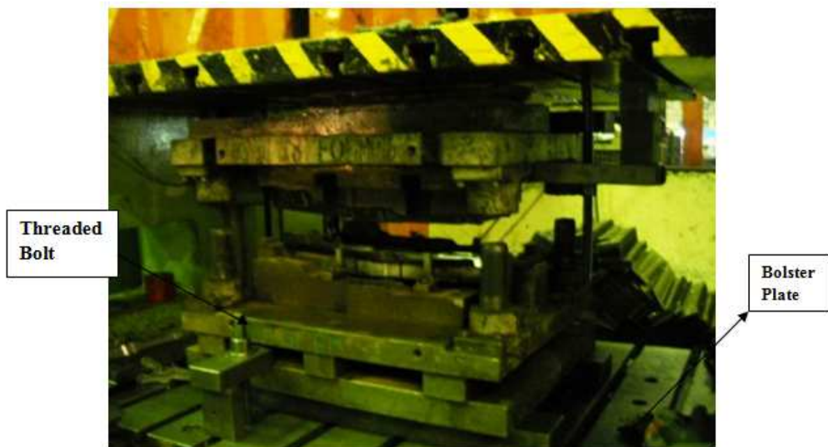
Figure7: Clamping of tool die at bolster with threaded bolt [Kansal Industries IMT Maneser]
