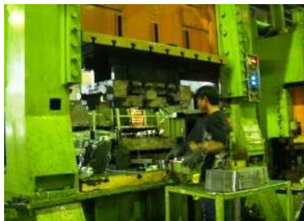
Figure 8: Shut heights setting with pneumatic gun [Kansal Industries IMT Maneser]
