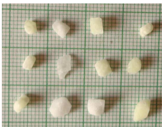
Figure 2. Optical photographs illustrating varied morphologies of Strontium tartrate crystals grown under different growth conditions
