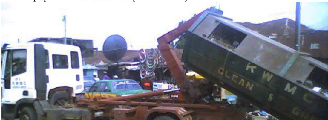
Plate 1: Dyno Truck lifting a Ro-Ro bin.
