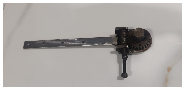
Figure 4: Elbow joint lock mechanism.
