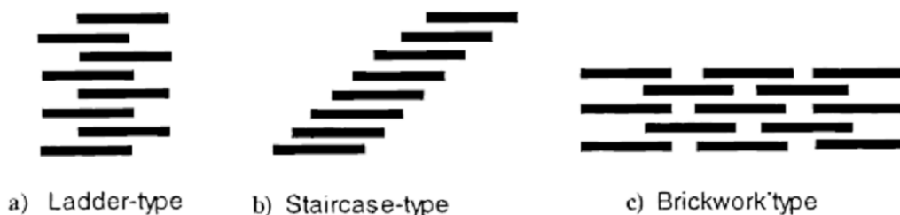
Fig1. Schematic representation of the different arrangement of cyanine dyes in the solid surface and in solution
