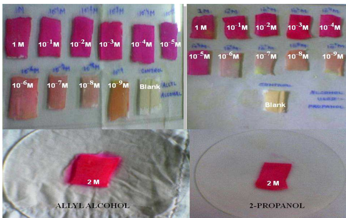
Fig.3:- Color of membranes prepared with different sol-gel 2-Propanol and Allyl Alcohol after reaction (Urea Solution 2\text{M} - 10^{-9}\text{M} )
