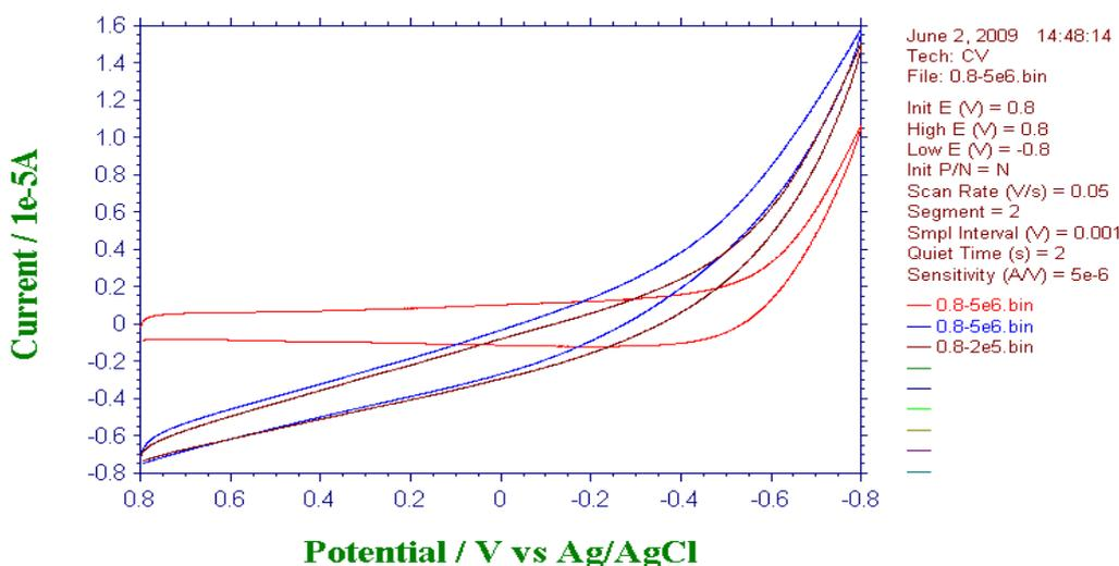
Figure 6: Cyclic voltammogram of buffer solution with Blank ITO and PdNP/ITO electrode via & 4Hr,12 Hr growth
