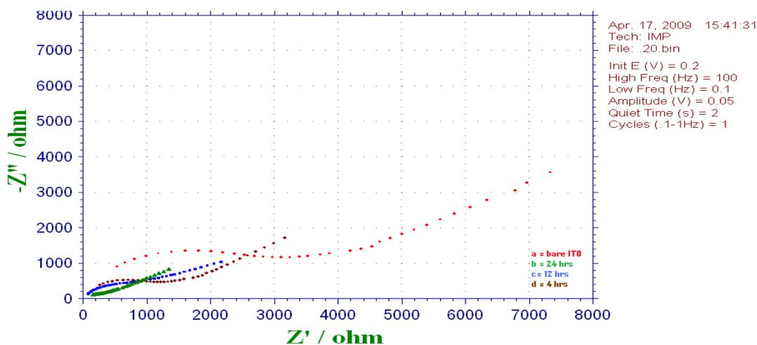
Figure 3: ECI Spectra in 1M KCl & 0.5mM Fe(CN)<sub>6</sub> solution with Bare ITO electrode and PdNP/ITO electrode prepared via 4 hr, 12 hr and 24 hr Growth
