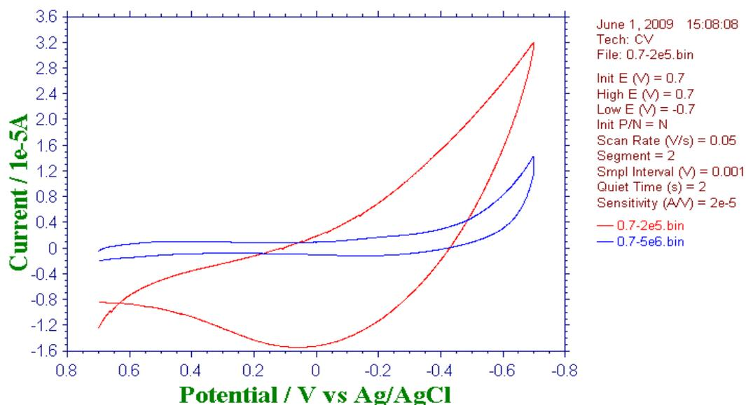
Figure 4: Cyclic Voltammogram of 1mM Fe(CN)<sub>6</sub> in Buffer Sol. (pH 7) with PdNP/ITO electrode via 2 hr Seed Solution immersion & 4 hr Growth in GS
