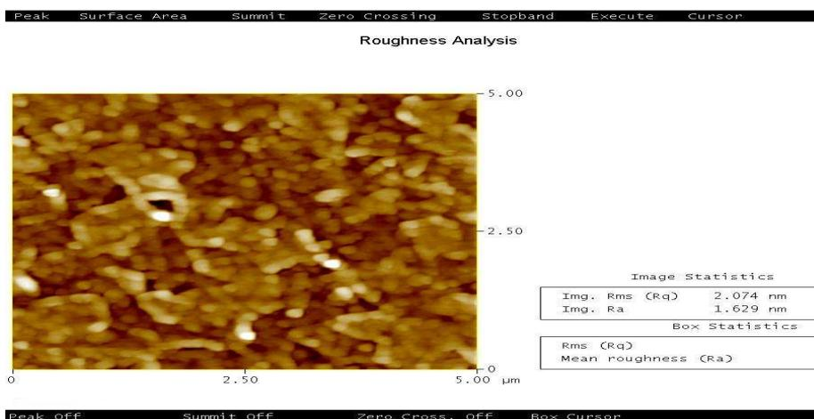
Figure 9: Roughness analysis of PdNPs after 12 hr growth
