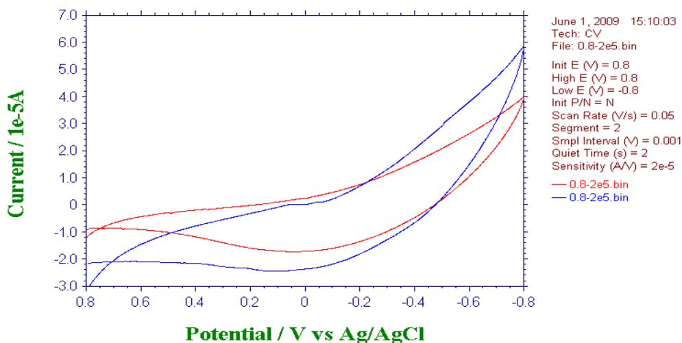
Figure 5: Cyclic Voltammogram of buffer solution with PdNP/ITO electrode via 4hr & 24hr growth
