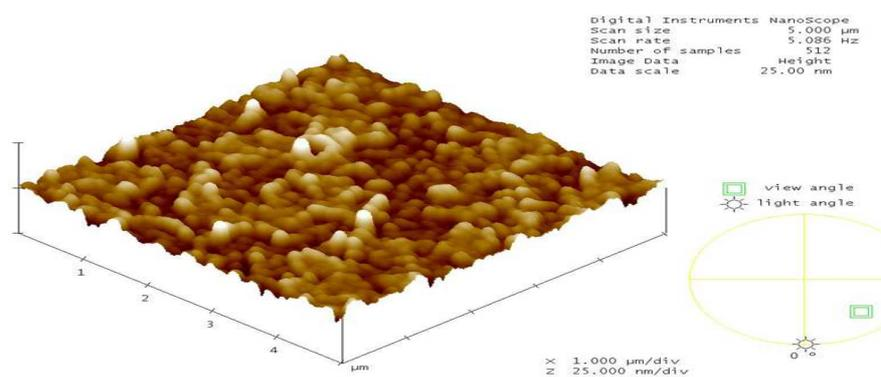
Figure 8: Typical 3-D image of PdNPs after 12 hr growth
