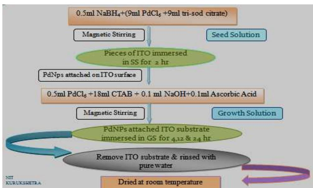
Figure 1: Synthesis Methodology of Pd Nanocrystals [21].
