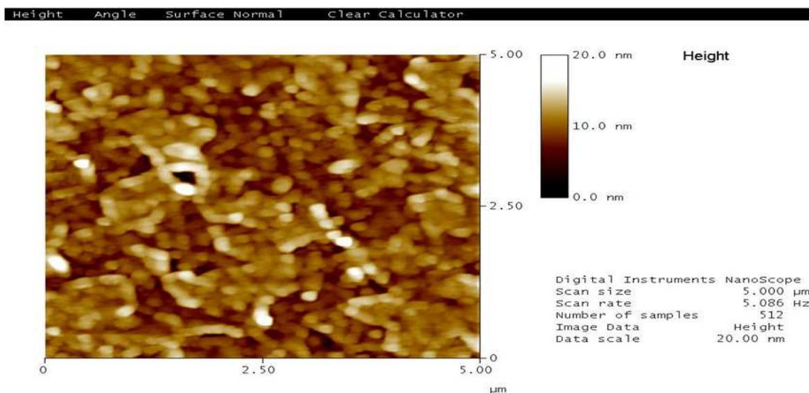
Figure 7: Typical AFM image of PdNPs after the 12 hr growth
