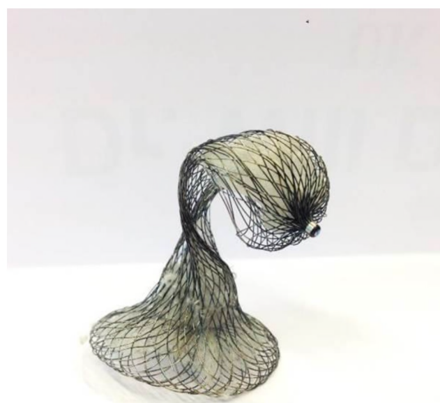
Figure 2 Cobra head conformation of the 16 mm Amplatzer Septal Occluder LA disc after retrieval, induced by manually twisting the device ex vivo
