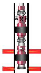
Figure 5 double seal single grip string schematic diagram
