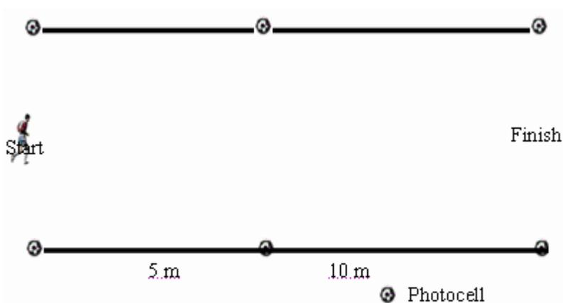
Figure 2. Acceleration test for 10 m. (9)
