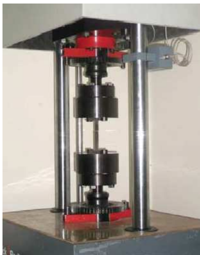
Figure 7: Fatigue testing of the laminate
