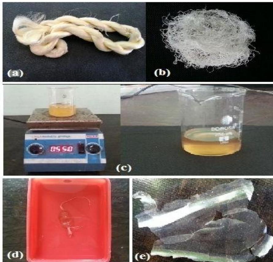
**Figure 1.** Shows (a) photograph of the silk fibers, (b) photograph of the silk fibers after the removal of sericine, (c) photograph of 5% silk solution dissolved in LiBr, (d) photograph of the dialysis set up against distilled water (e) silk films obtained
