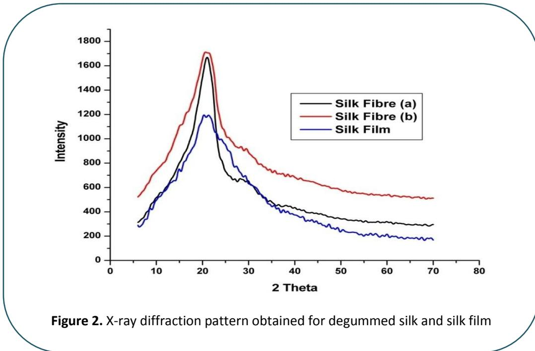
Figure 2. X-ray diffraction pattern obtained for degummed silk and silk film
