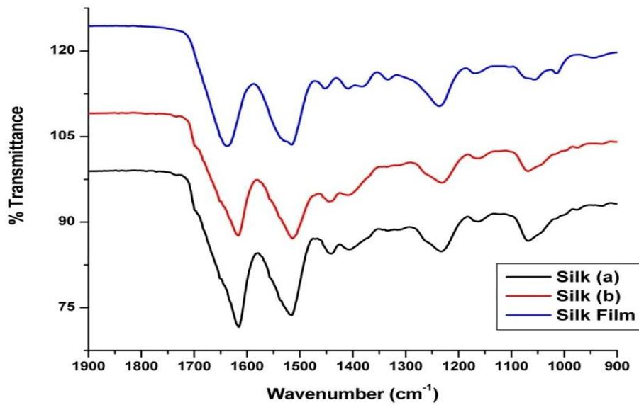
**Figure 4.** FTIR spectra of silk fiber (a), degummed silk fiber (b) and silk film
