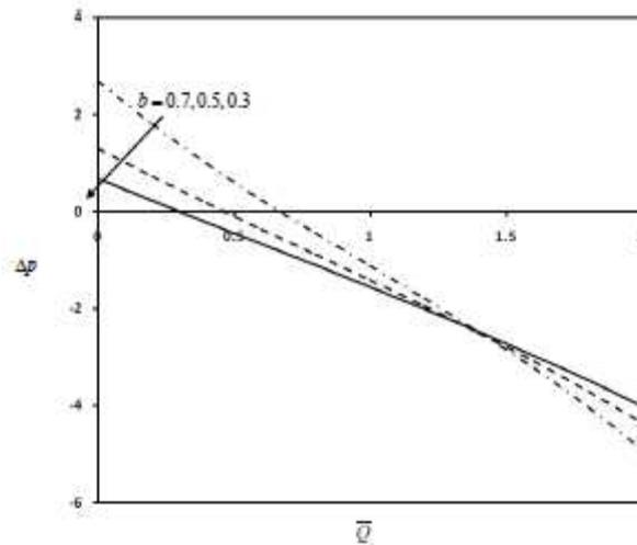
Fig. 7. The variation of pressure rise  $\Delta p$  with time averaged flux  $\bar{Q}$  for different values of lower wave amplitude  $b$  with  $\alpha = 0.5, \Gamma = 0.01, M = 1, \theta = \frac{\pi}{4}$  and  $d = 1.2$ .
