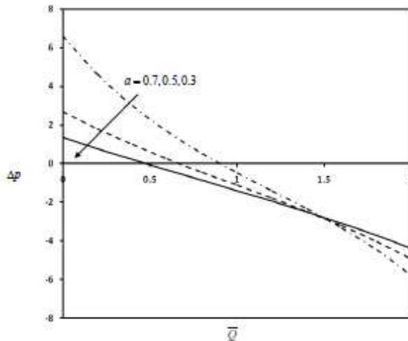
Fig. 6. The variation of pressure rise  $\Delta p$  with time averaged flux  $\bar{Q}$  for different values of upper wave amplitude  $\alpha$  with  $\Gamma = 0.01, \delta = 0.7, M = 1, \theta = \frac{\pi}{4}$  and  $d = 1.2$ .
