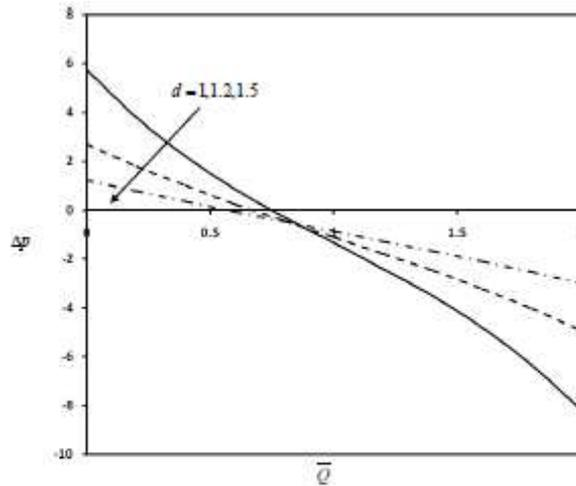
Fig. 5. The variation of pressure rise  $\Delta p$  with time averaged flux  $\bar{Q}$  for different values of  $d$  with  $a = 0.5, b = 0.7, M = 1, \theta = \frac{\pi}{4}$  and  $\Gamma = 0.01$ .
