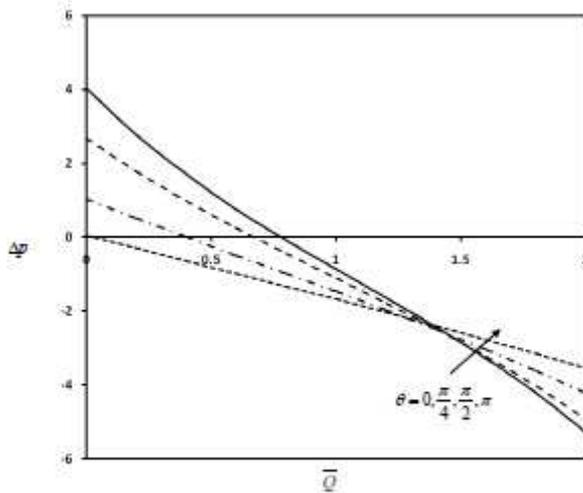
Fig. 4. The variation of pressure rise  $\Delta p$  with time averaged flux  $\bar{Q}$  for different values of phase shift  $\theta$  with  $a = 0.5, b = 0.7, M = 1, \Gamma = 0.01$  and  $d = 1.2$ .
