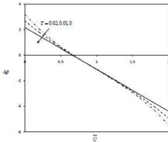
Fig. 2. The variation of pressure rise  $\Delta p$  with time averaged flux  $\bar{Q}$  for different values of Deborah number  $\Gamma$  with  $a = 0.5, b = 0.7, M = 1, d = 1.2$  and  $\theta = \frac{\pi}{4}$ .
