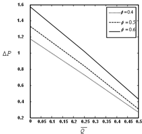
Fig.12: Variation of pressure rise versus mean flow rate for different  $\phi$
