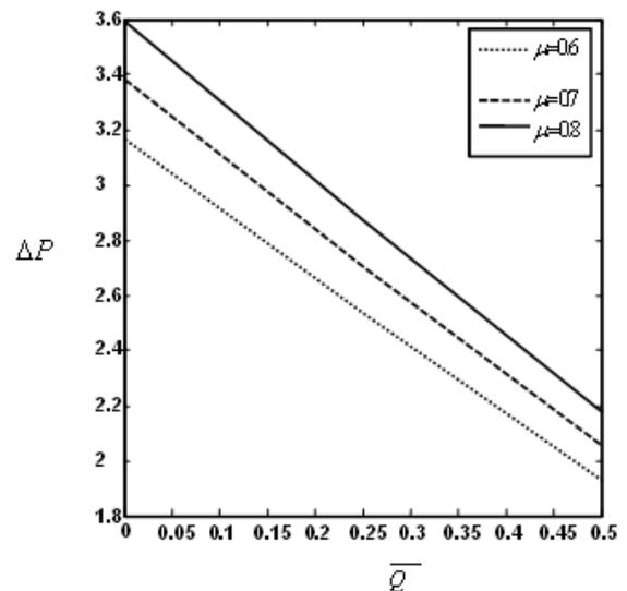
Fig.9: Variation of pressure rise versus mean flow rate for different  $\mu$  ( $M_1=1.5, M_2=1$ ) with fixed  $\gamma=0.4, \phi=0.6, \epsilon=0.4, Da=0.6$
