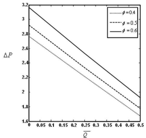
Fig.13: Variation of pressure rise versus mean flow rate for different  $\phi$  with fixed  $M_1=1.5, M_2=1, \gamma=0.4, \mu=0.6, \epsilon=0.4, Da=0.6$ .
