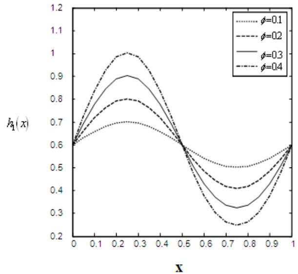
Fig.7: The Shape of the interface for different  $\phi$  with fixed  $M_1=1.5, M_2=1, \gamma=0.6, \mu=2, \epsilon=0.5, Da=0.5, Q=0.5$ .
