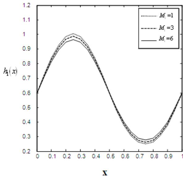
Fig.4: The Shape of the interface for different  $M_1$  with fixed  $M_2=1, \gamma=0.6, \phi=0.4, \epsilon=0.5, Da=0.5, \mu=2, Q=0.5$ .
