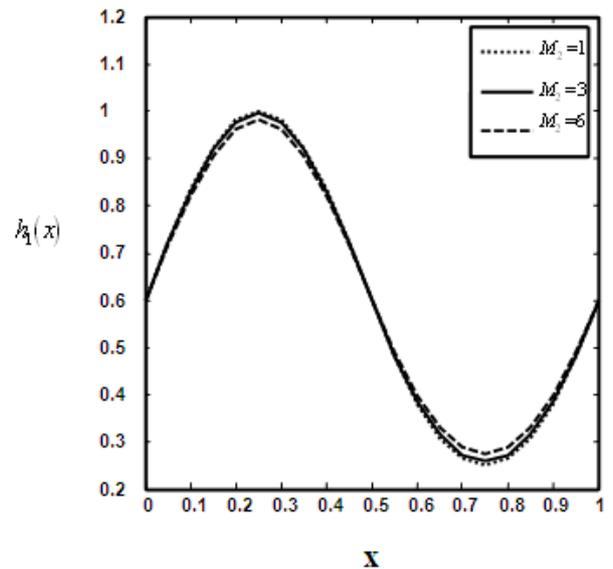
Fig.5: The Shape of the interface for different  $M_2$  with fixed  $M_1=1, \gamma=0.6, \phi=0.4, \epsilon=0.5, Da=0.5, \mu=2, Q=0.5$ .
