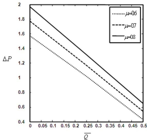
Fig.8: Variation of pressure rise versus mean Flow rate for different  $\mu$  ( $M_1=0.5, M_2=1$ ).
