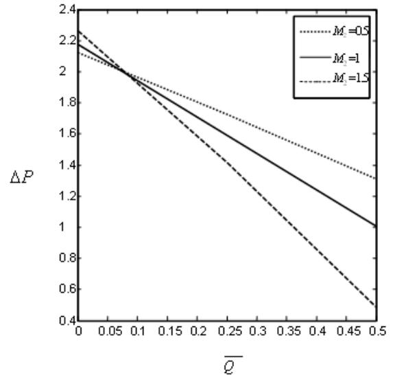
Fig.11: Variation of pressure rise versus mean flow rate for different  $M_2$  ( $M_1=1$ ) with fixed  $\gamma=0.4, \phi=0.6, \epsilon=0.4, Da=0.6, \mu=0.6$ .
