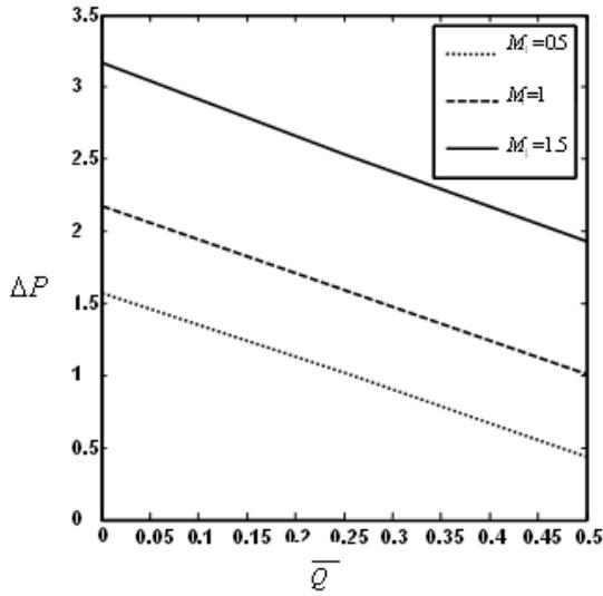
Fig.10: Variation of pressure rise versus mean flow rate for different  $M_1$  ( $M_2=1$ ).
