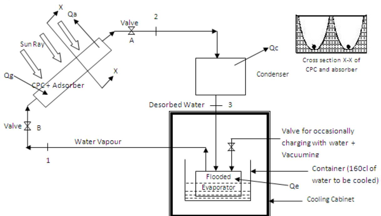
Figure 1; Adsorption Refrigerator Design flow diagrams
