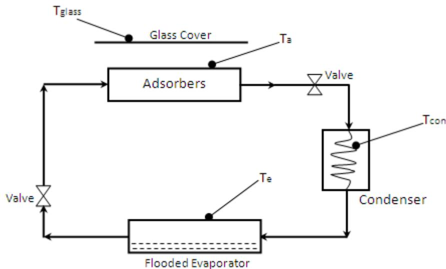
Figure 2: Flow diagram and Instrumentation
