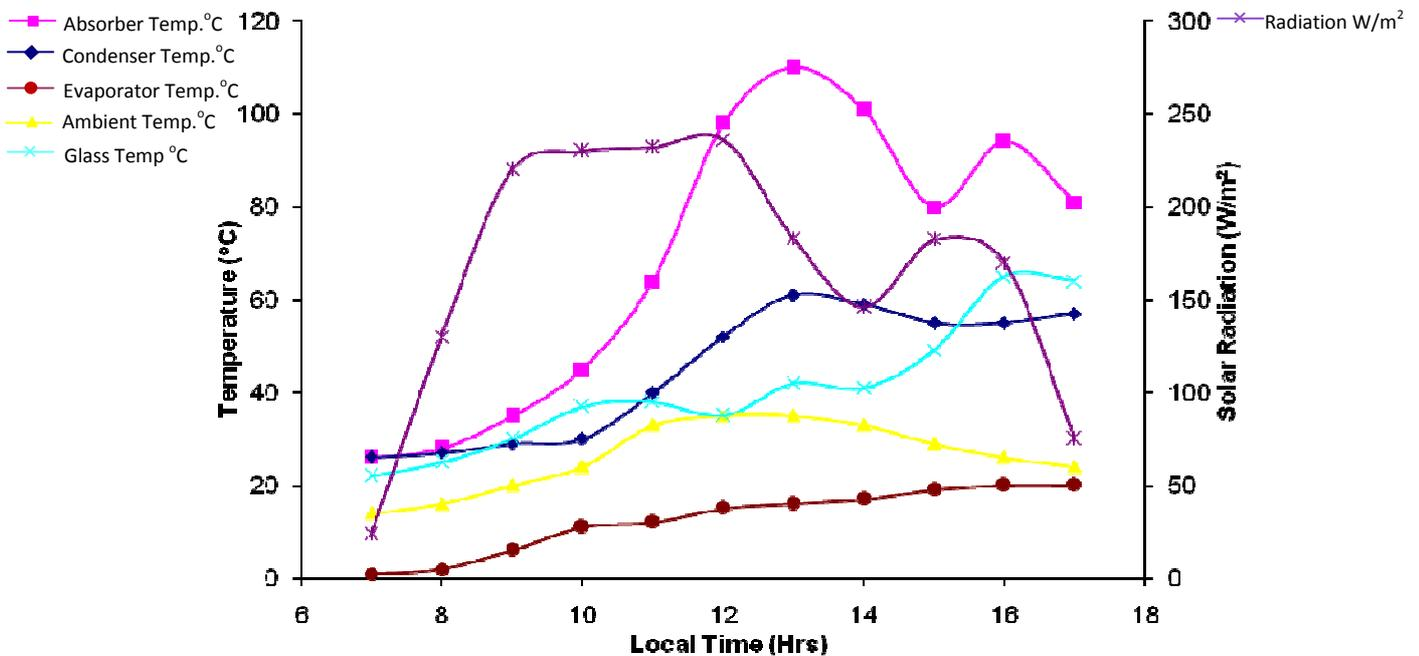
Figure 3: Day 1(1<sup>st</sup>April 2011) Hourly variation of Solar Radiation and system temperature in a day
