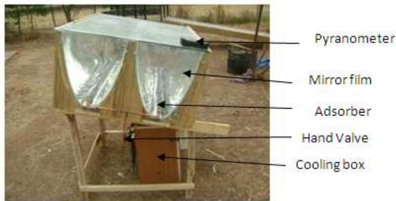
Plate 1; System assembly (Side view)
