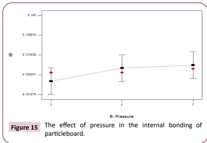
**Figure 15** The effect of pressure in the internal bonding of particleboard.
