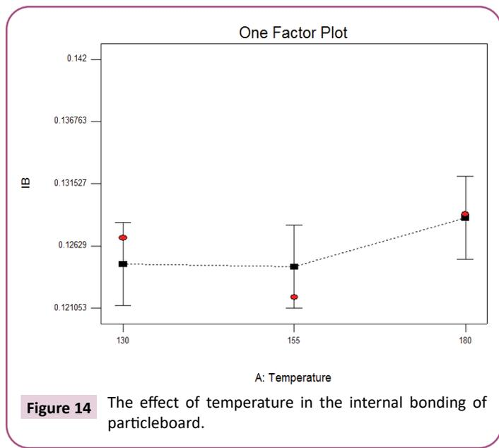
**Figure 14** The effect of temperature in the internal bonding of particleboard.
