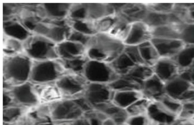
**Figure 3** Typical microstructure of layer I of corncob in 400  $\mu\text{m}$ .
