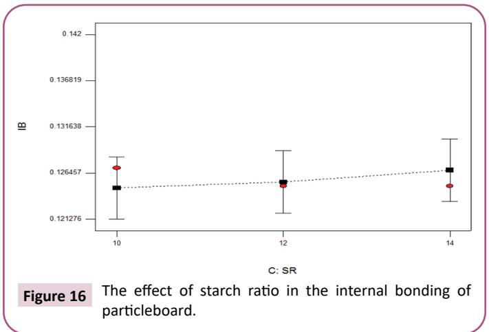
**Figure 16** The effect of starch ratio in the internal bonding of particleboard.
