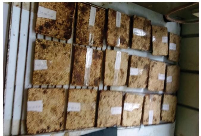
Figure 10 Experimental products of maize cob particle board.
