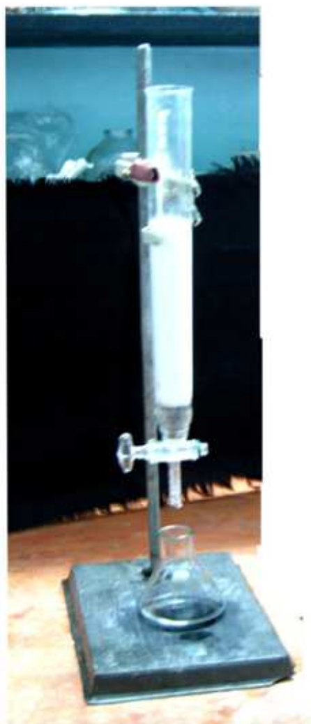
Figure II : Purification of Dialysed Enzymes by Ion Exchange Chromatography
