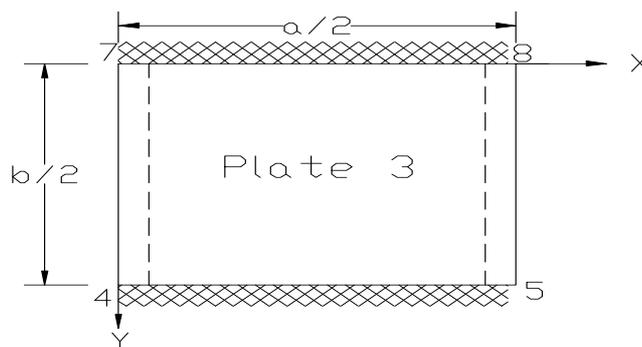
Fig. 6: Assumed Support Condition for Plate 3
