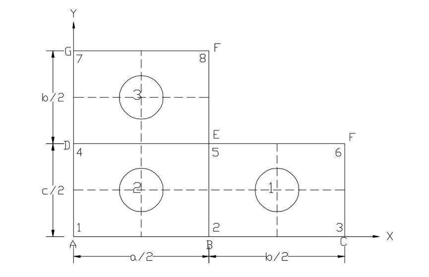
Fig.3: Flat plate idealization of one-eighth of a box (shown in Fig. 2.)
