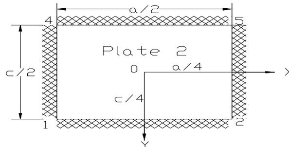
Fig. 5: Assumed Support Condition for Plate 2
