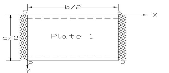
Fig. 4 Assumed support condition for plate 1
