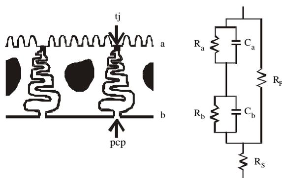
**Figure 4.** Equivalent electric circuit used to obtain estimates of the apical and basolateral membrane resistances ( $R$ ) and capacitances ( $C$ ) by impedance analysis.
