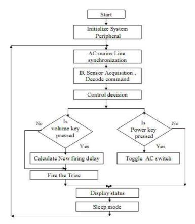
Fig.4. The basic flow chart of the device software
