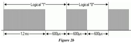
Fig. 2.IR transmitter protocol
