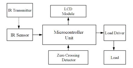
Fig.1. Hardware Block Diagram
